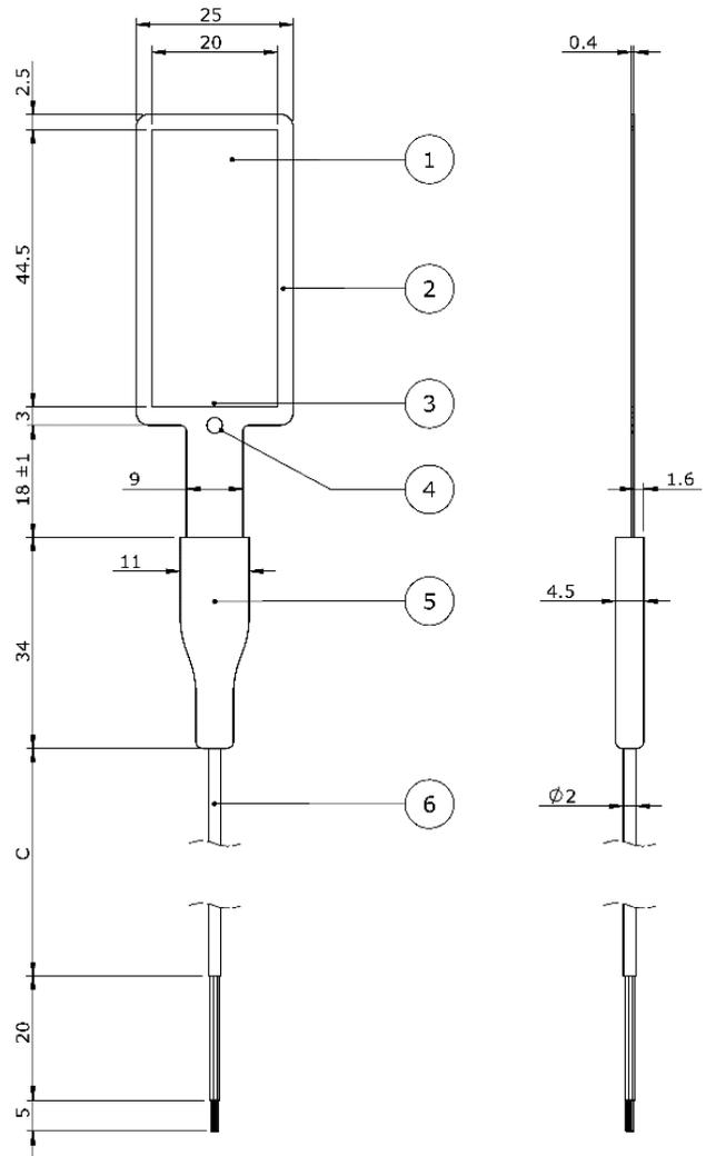
**Figure 4** FHF06 high temperature foil heat flux sensor: (1) sensing area with thermal spreaders, (2) passive guard area with thermal guard, (3) type T thermocouple, (4) dot indicating front side, (5) cable connection block for strain relief, (6) cable, standard length is 2 m. Can be 2, 5 or 10 m. All dimensions in  $\times 10^{-3}$  m.
