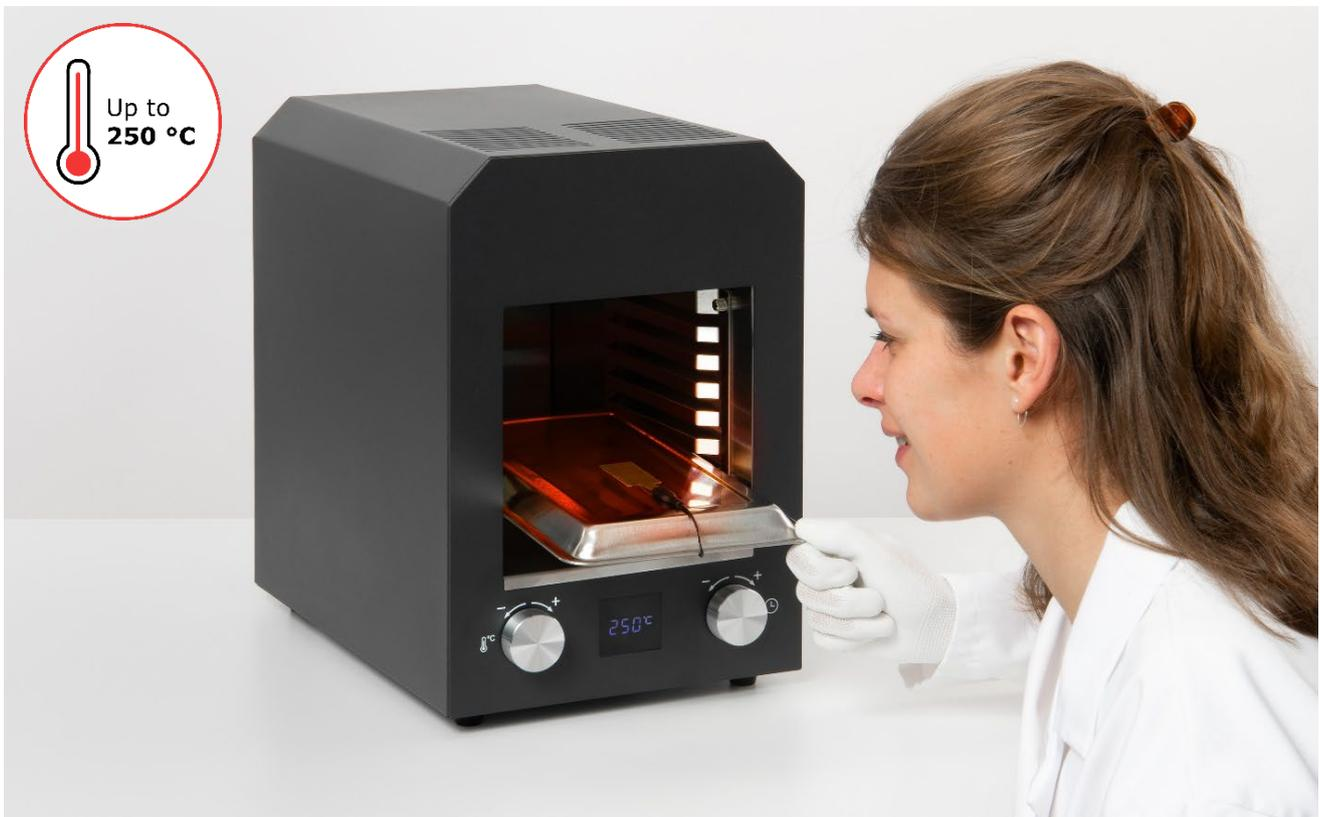
**Figure 1** FHF06 high temperature foil heat flux sensor being used to monitor the performance of an oven. The sensor is suitable for use under continuous exposure to temperatures up to 250 °C.
