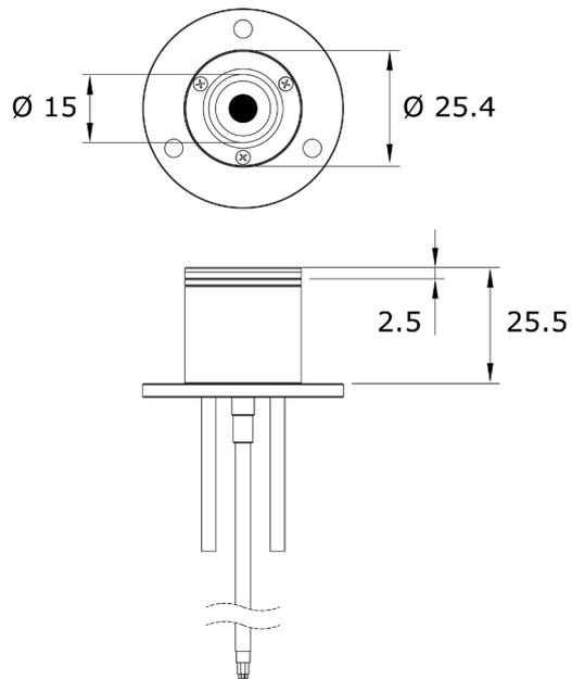
**Figure 3.3.1** GG01 with sapphire window, dimensions in  $10^{-3}$  m. The window is added to a standard GG01. GG01s with sapphire window (GG01-250-SW) are custom made, the sapphire window cannot be used on a standard GG01. For other dimensions, see previous section on GG01 dimensions
