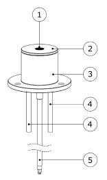
**Figure 3** overview of GG01 standard model: (1) Gardon gauge sensor with black coating, (2) copper housing, (3) sensor body with flange, (4) water cooling tubes, (5) cable; standard cable length is 2 m
