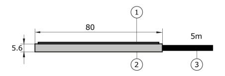
**Figure 3.1.1** *HFP01SC* heat flux sensor dimensions in x 10<sup>-3</sup> m
