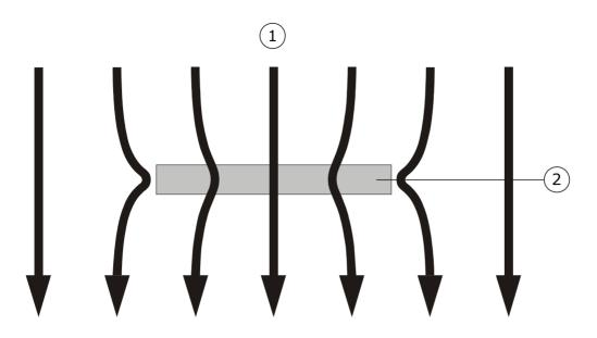
**Figure 6.3.3.1** the deflection error. The heat flux (1) is deflected in particular at the edges of the sensor. The measurement will contain an error; the so-called deflection error. The magnitude of this error depends on the thermal conductivity of the environment, sensor thermal conductivity as well as sensor design and contact resistance.
