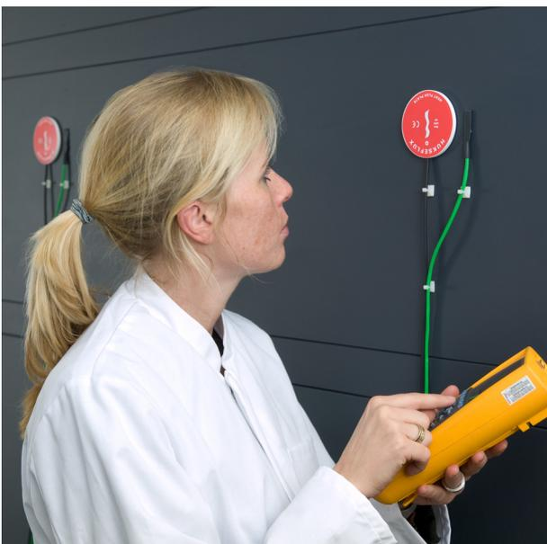
**Figure 2** HFP01 heat flux sensor in use
