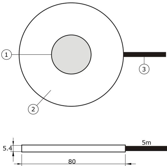
**Figure 3** HFP01 heat flux plate: (1) sensing area, (2) passive guard of ceramics-plastic composite (3) cable, standard length is 5 m. Total sensor thickness including covers is  $5.4 \times 10^{-3}$  m. Dimensions in  $\times 10^{-3}$  m
