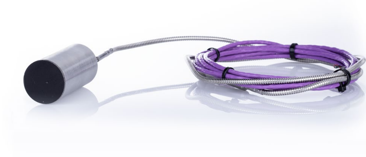
Figure 1.2.1 HFS01 showing its metal body, black coating and cable. The removable flange is included but not pictured here.
