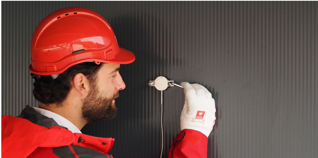
Figure 0.3 IHF01 industrial heat flux sensor mounted on a wall using tack-welded threads and spring-loaded bolts.
