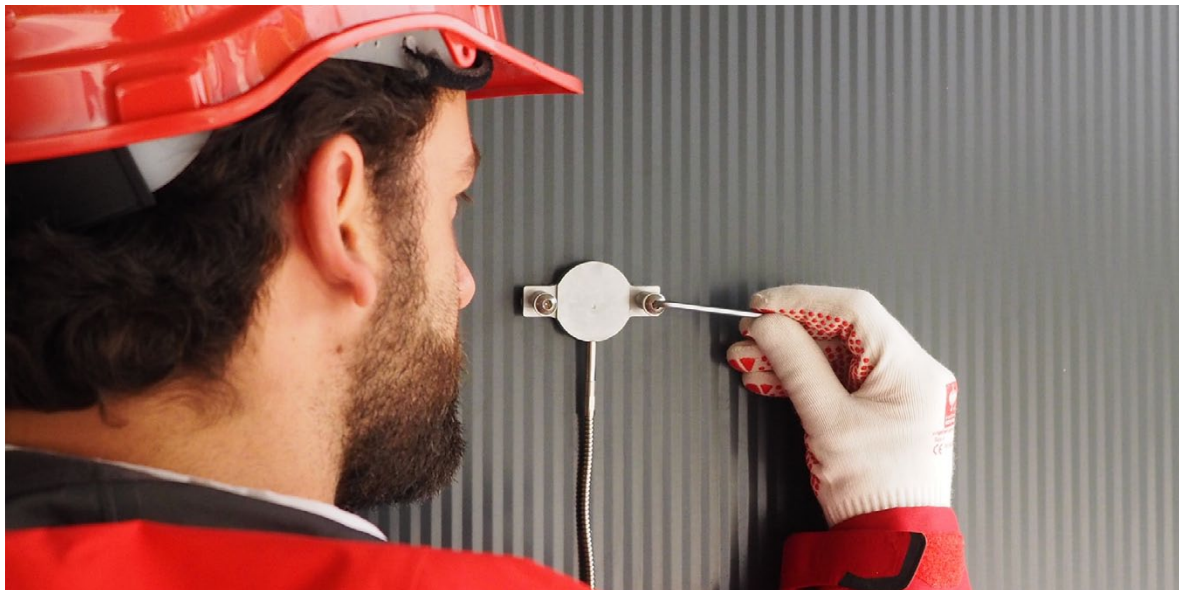
Figure 4.1.1 Example of an IHF01 industrial heat flux sensor mounted on a wall using spring-loaded bolts and tack-welded threads. The sensor is mounted on a well prepared flat surface.
