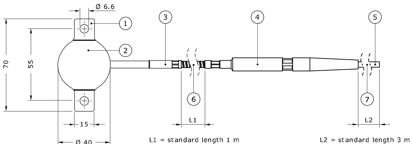
**Figure 4** IHF01: the heat flux sensor consist of a stainless steel body (1) which is connected via a rigid stainless steel coupler (3) to a flexible high-temperature metal sheathed cable with interlocked spiral stainless steel armour (6). After a transition piece (4), wires are extended using a low-temperature extension cable (7). In the standard configuration, the cable ends in bare wires (5). Two mounting flanges (2) are attached to the body. Dimensions in  $\times 10^{-3}$  m.
