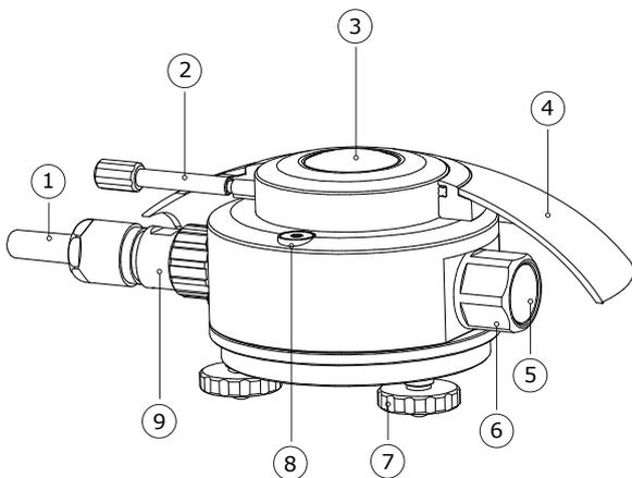
**Figure 2** overview of IR20 pyrgometer:
