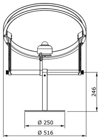
Figure 3 SHR02 dimensions in  $\times 10^{-3}$  m
