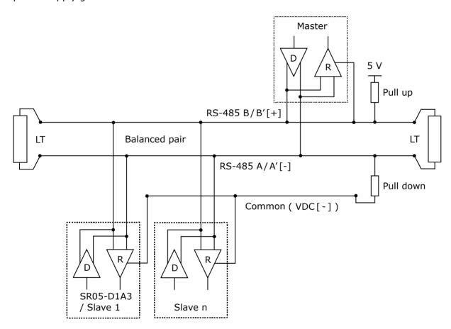
**Figure 5.10.1** Typical topology of a two-wire RS-485 network, figure adapted from: Modbus over serial line specification and implementation guide V1.02 (www.modbus.org). The power supply is not shown in this figure.
