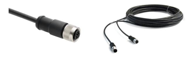
**Figure 9.1.1** On the left the SR05 cable with M12-A female connector on sensor end. The cable is non-stripped on the other end. Its length is 3 metres standard and available in 10 and 20 metres too. On the right Hukseflux extension cable with connector pairs, with male and female M12-A connectors, available in 10 and 20 metres.
