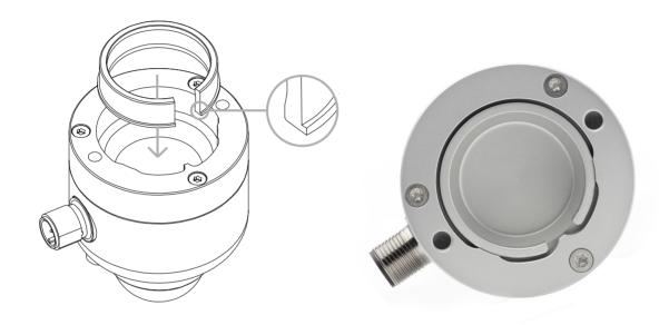
**Figure 5.4.1.1** Line drawing indicating placement of the aluminium shim and photo showing the shim properly positioned in the centre of SR05's bottom plate. Note the position of the protruding ledge when placing the shim.
