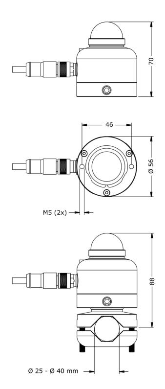
**Figure 3.2.1** Dimensions of SR05 in  $\times$  10<sup>-3</sup> m. The bottom drawing shows the height of SR05 combined with its optional ball levelling mount and the tube diameter required for use with SR05's optional tube mount. M5 mounting bolts and the countersunk set screw require a 4 mm hex key for mounting and levelling.
