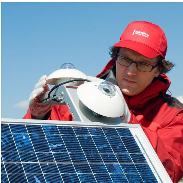
**Figure 2** PV system performance monitoring pyranometers
