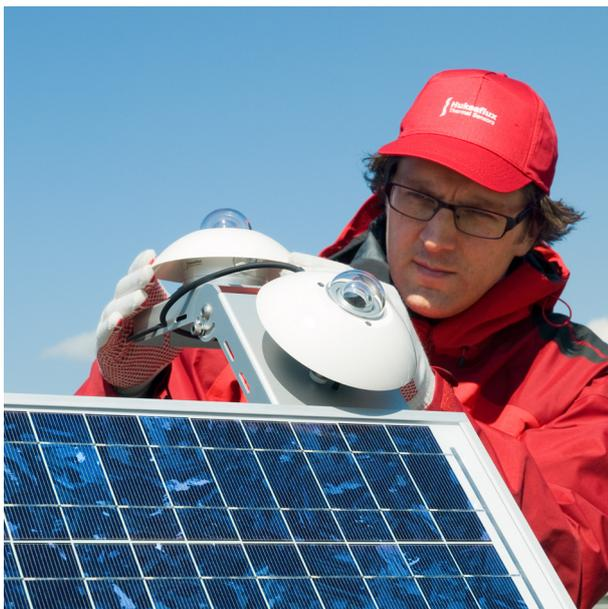
**Figure 2** PV system performance monitoring pyranometers
