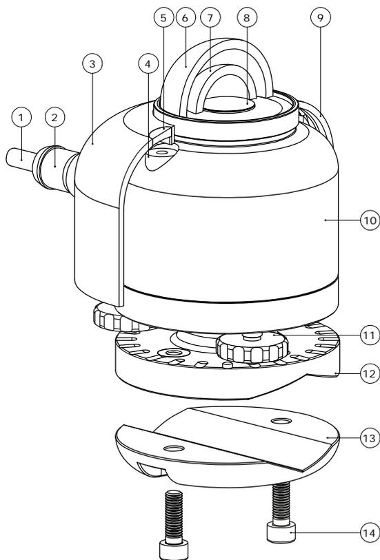
**Figure 3** overview of SR15-A1: (1) cable, (2) connector, (3) sun screen, (4) bubble level, (5) bubble level window, (6) outer dome, (7) inner dome, (8) thermal sensor with black coating, (9) quick release system of sun screen, (10) instrument body, (11) levelling feet, (12) optional spring-loaded levelling mount, (13) optional tube mount, (14) screws included with tube mount
