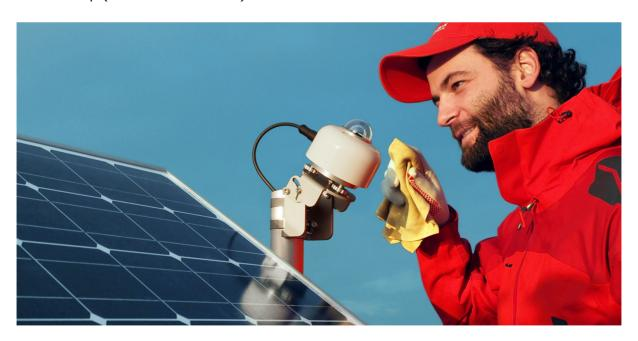
**Figure 0.2** SR15 pyranometer mounted on a mast in PoA (Plane Of Array) for PV system performance monitoring
