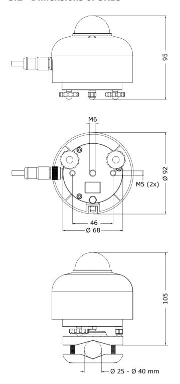
**Figure 3.2.1** Dimensions of SR15 in  $\times$  10<sup>-3</sup> m. Mounts are optional
