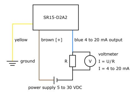
**Figure 5.8.2** Electrical diagram of the connection of SR15-D2A2 to a typical voltmeter or datalogger with the capacity to measure voltage signals. Usually a 100  $\Omega$  shunt resistor (R) is used to convert the current to a voltage. SR15-D2A2 operates on a supply voltage of 5 to 30 VDC.
