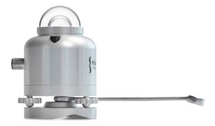
**Figure 5.3.1.4** SR15 levelling mount seen from the side: (un)locking with a 10 mm spanner
