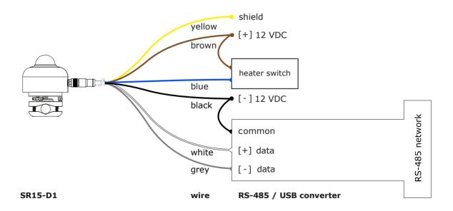
**Figure 5.10.3** Connection of SR15-D1 to an RS-485 network. SR15-D1 is powered by an external power supply of 12 VDC. The heater is powered by the same power supply, and is optionally switches on or off by an external switch.
