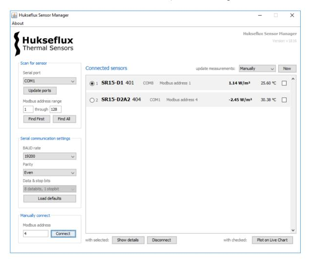
Figure 6.1.3.2 Sensor Manager main window with two connected SR15's
