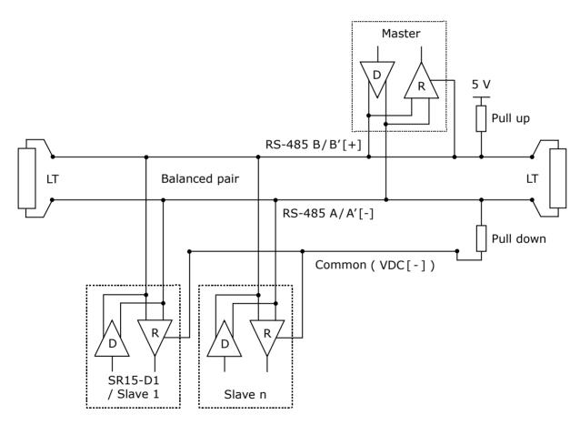
**Figure 5.10.1** Typical topology of a 2-wire RS-485 network, figure adapted from: Modbus over serial line specification and implementation guide V1.02 (www.modbus.org). The power supply is not shown in this figure.
