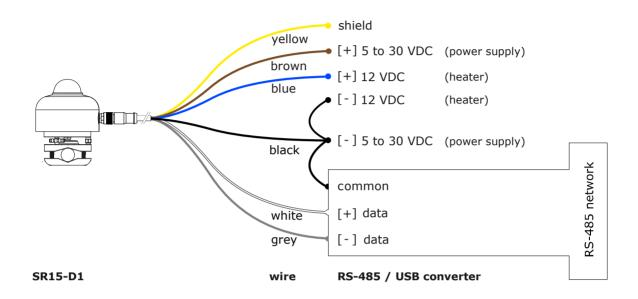
**Figure 5.10.2** Connection of SR15-D1 to an RS-485 network. SR15-D1 is powered by an external power supply of 5 to 30 VDC. The heater is powered by a different power supply with a recommended voltage of 12 VDC.
