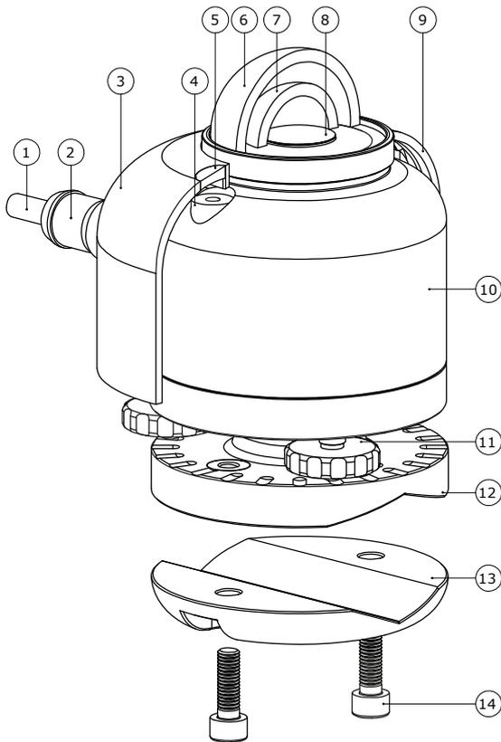
**Figure 3** Overview of SR15: (1) cable, (2) connector, (3) sun screen, (4) bubble level, (5) bubble level window, (6) outer dome, (7) inner dome, (8) thermal sensor with black coating, (9) quick release system of sun screen, (10) instrument body, (11) levelling feet, (12) optional spring-loaded levelling mount, (13) optional tube mount, (14) screws included with tube mount.
