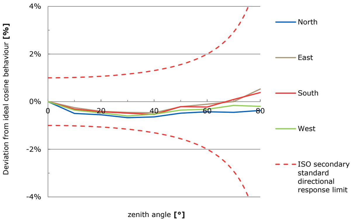
**Figure 2.3** Directional response of a SR20 pyranometer of 4 azimuth angles, compared to secondary standard limits
