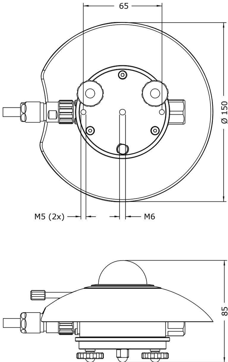
**Figure 3.2.1** Dimensions of SR20 in  $\times 10^{-3}$  m.
