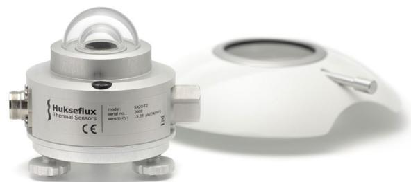
**Figure 5** SR20 with its sun screen removed.
