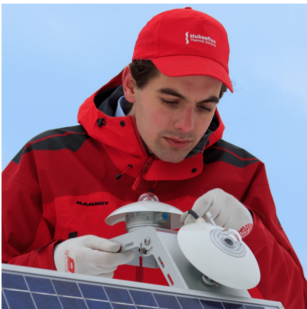
Figure 2 Dual setup in PV system performance monitoring.
