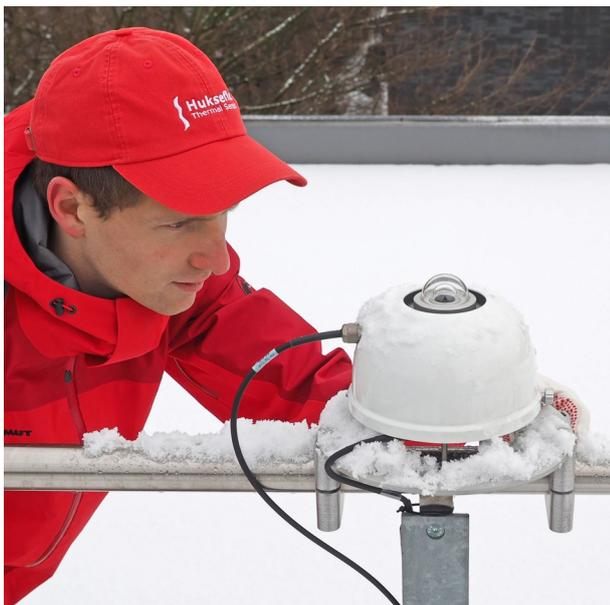
**Figure 2** SR22 sensor combined with VU01 ventilation unit
