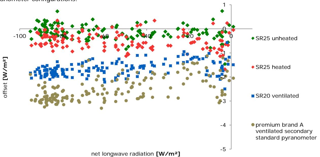
**Figure 3** results at Hukseflux: nighttime offsets of ventilated pyranometers and SR25 versus net longwave radiation. SR25 has lower nighttime offset than the ventilated secondary standard pyranometers both when unheated and when heated
