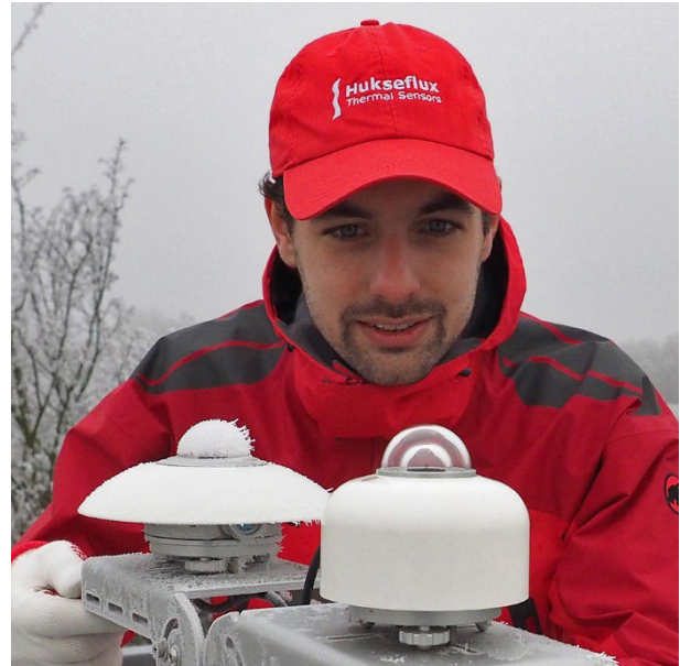
Figure 4 Heated to counter frost and dew deposition: clear difference between a non-heated pyranometer (back) and SR30 with RVH™ technology (front).
