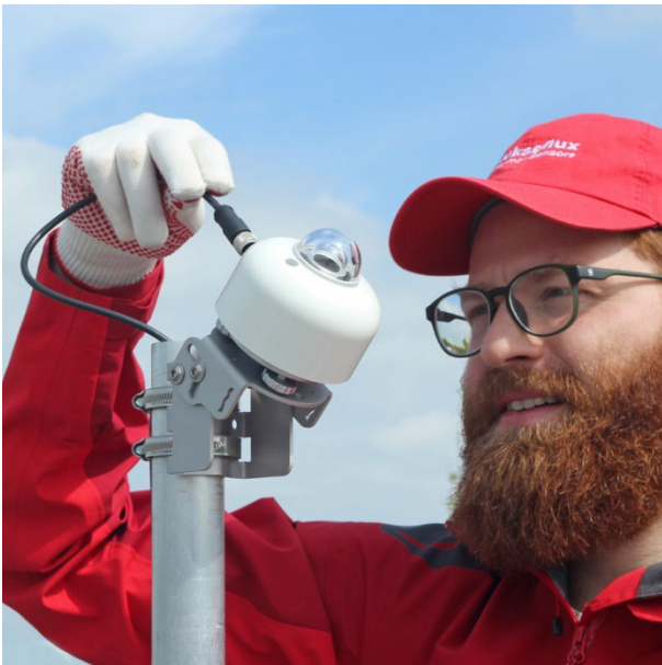
Figure 10 PMF01 pyranometer mounting fixture can be used for easy installation of a pyranometer in Plane of Array for PV system performance monitoring.
