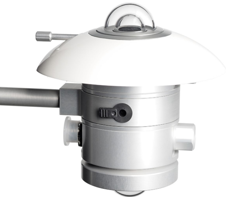
Figure 1 SRA20-D2 Class A albedometer.
