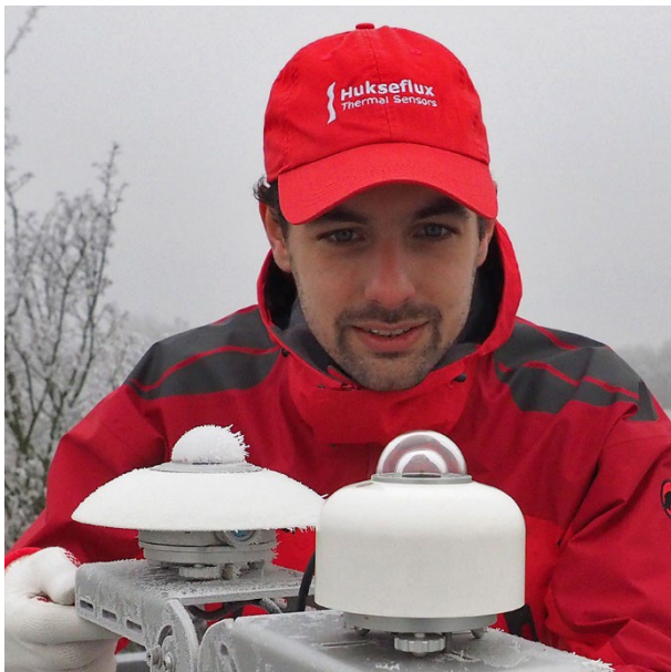
Figure 2 Heated to counter frost and dew deposition: clear difference between a non-heated pyranometer (back) and SR30 with RVH™ technology (front).
