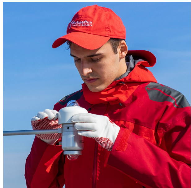
Figure 5 Using the SRA30 albedometer is easy; the instrument is composed of AMF03 and two SR30-M2-D1 pyranometers.
