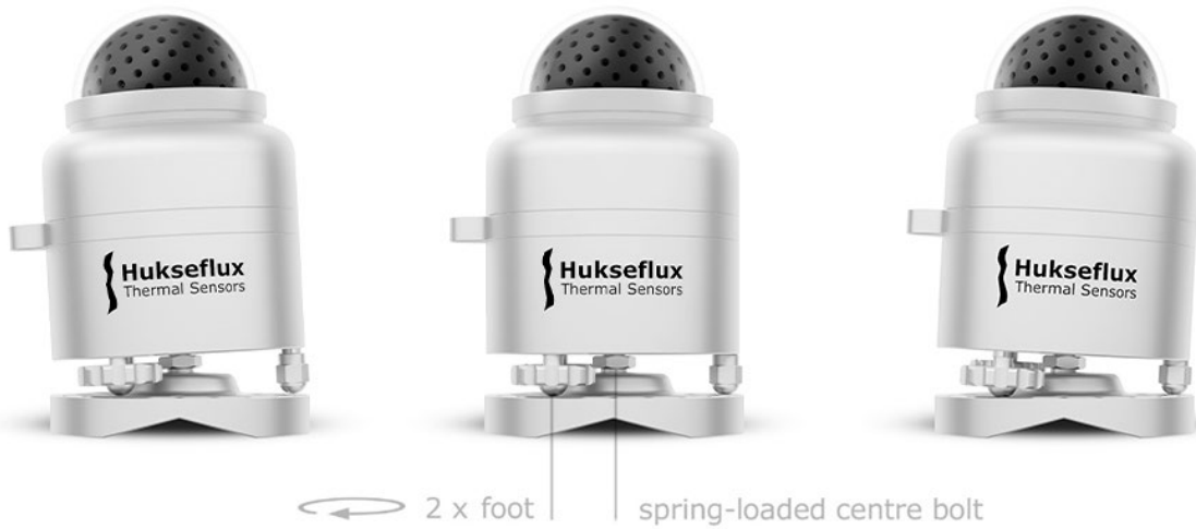
Figure 0.8 LM01 levelling mount is the most popular option for SRD100-D1: practical spring-loaded mount for easy mounting, levelling and instrument exchange on flat surfaces. The spring-loaded mounting has the advantage that levelling can be done quickly, without unlocking the instrument.
