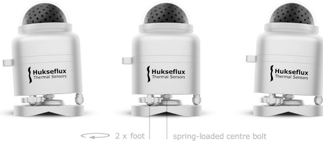
Figure 5.3.4.1.5 SRD100-D1 locked on its optional levelling mount: by fastening (on the left) or loosening (on the right) the two adjustable feet, the pyranometer can be levelled, using the bubble level as a reference. The static foot remains fixed. In all cases, ensure the legs of the pyranometer fit into one of the small ledges of the levelling mount. Locking is in place, when the nut is turned all the way against the bottom plate of the pyranometer.
