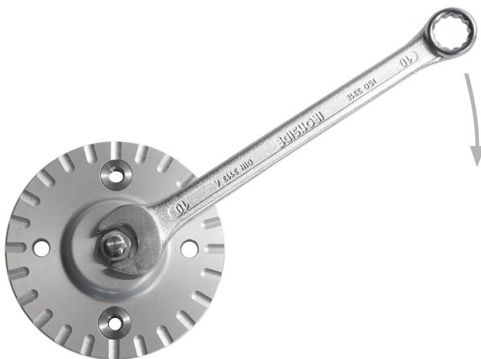
Figure 5.3.4.1.3 LM01 levelling mount seen from above: (un)locking with a 10 mm spanner.
