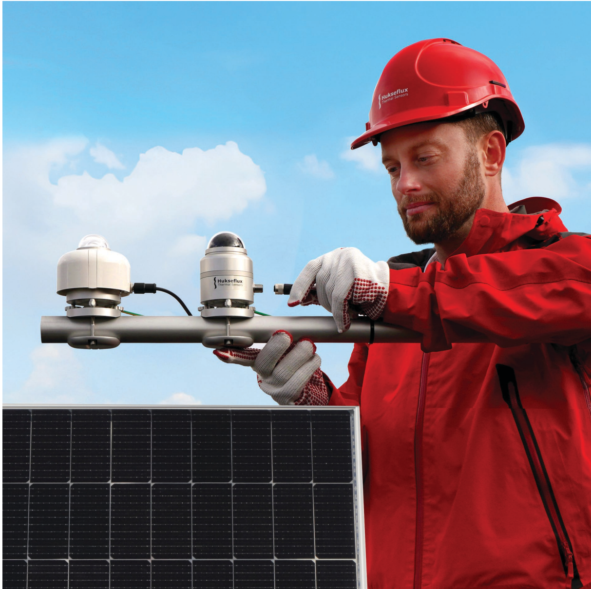
Figure 0.3 Typical installation of SRD100, next to a normal Class A pyranometer, such as the SR300-D1.
