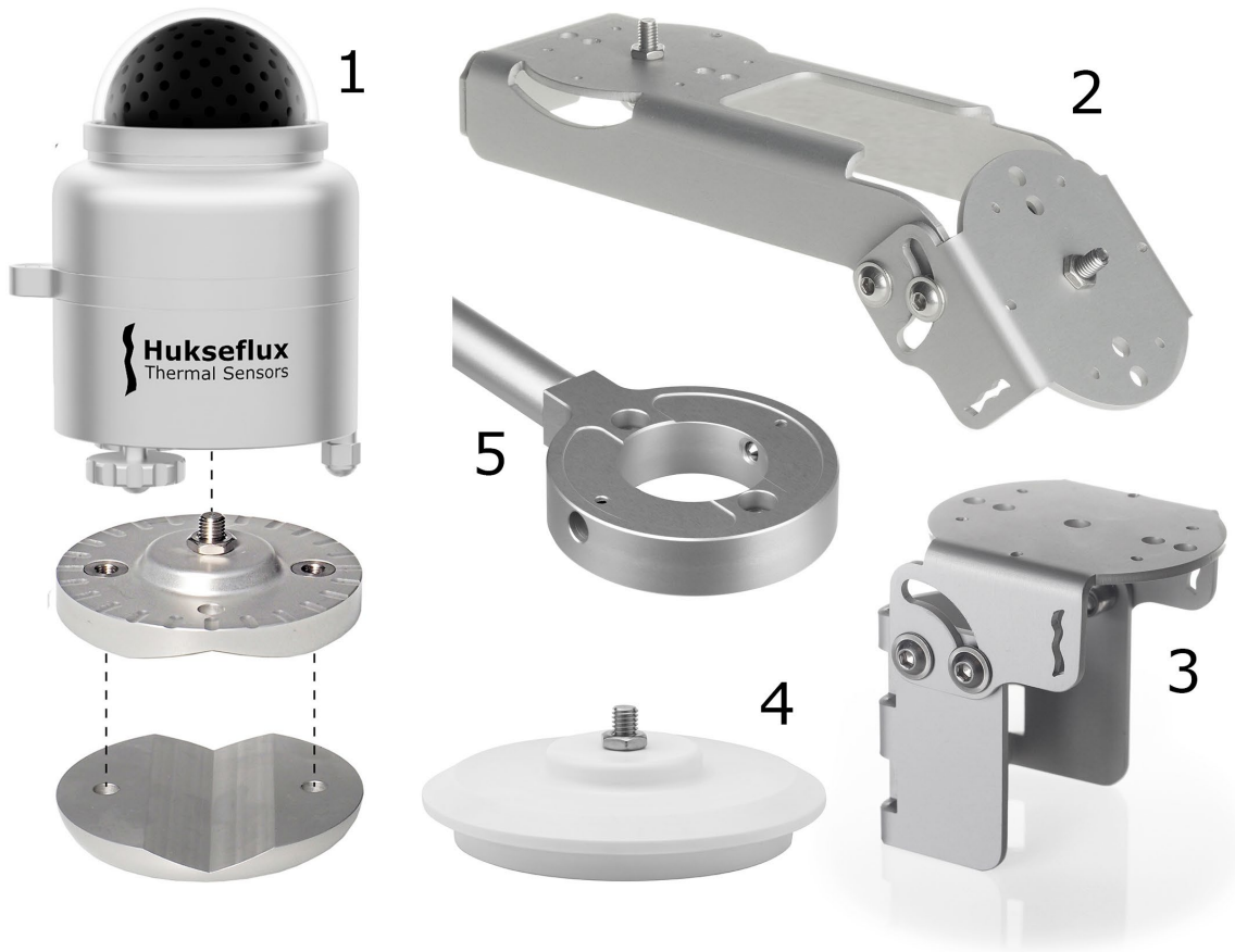
Figure 5.3.4.1 Overview of Hukseflux mounting options. 1. TLM01, 2. PMF02, 3. PMF01, 4. PID01, 5. AMF01.
