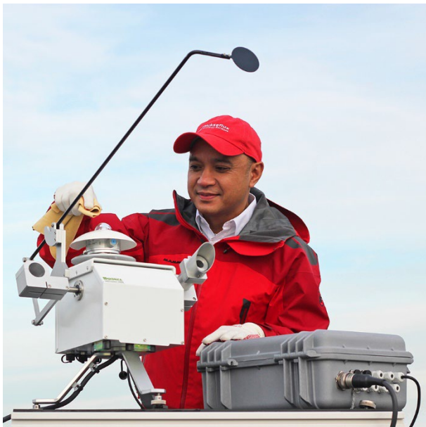
Figure 5 A traditional solution for diffuse and direct solar radiation measurement: an automated, motor-driven dual-axis solar tracker equipped with a pyrheliometer and shaded pyranometer. SRD100 offers a low-maintenance and more robust (no-moving parts) alternative.
