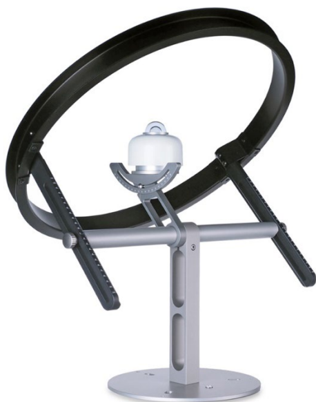
Figure 4 A traditional method for diffuse radiation measurement: using a pyranometer with a shadow ring. SRD100 offers a low-maintenance alternative.
