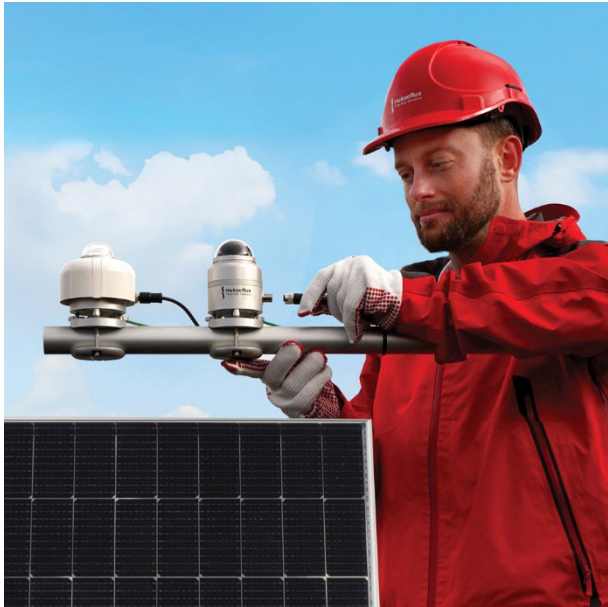
Figure 3 Typical installation of SRD100, next to a normal Class A pyranometer, such as the SR300-D1.
