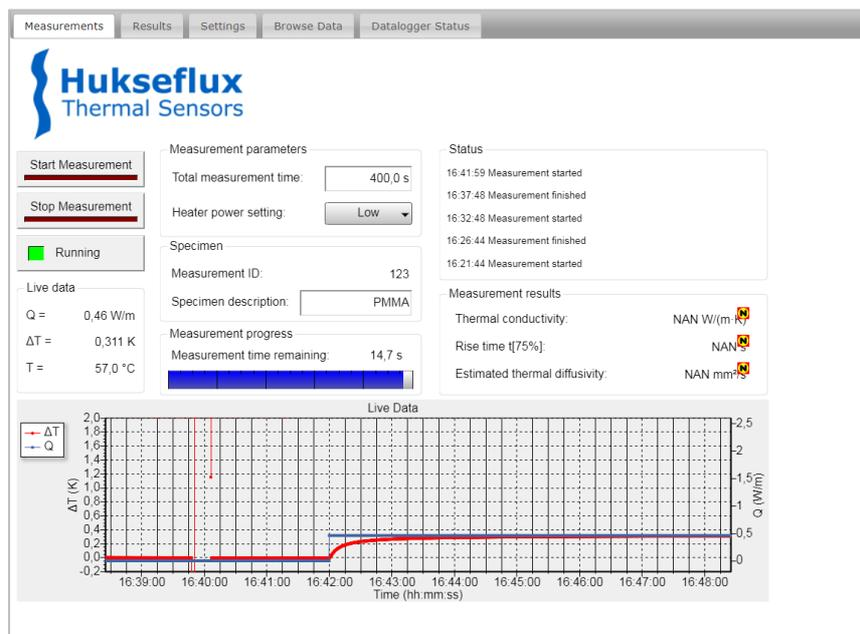
**Figure 0.4** STPSYS05's user interface: the main screen is used to start measurements, display live data and results
