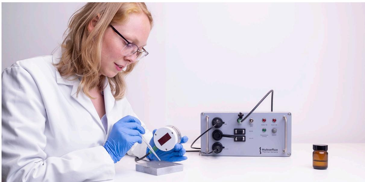
**Figure 5.1.2.1:** Place a drop of glycerol on the surface of the specimen in order to ensure optimal thermal contact between the specimen and the sensor.
