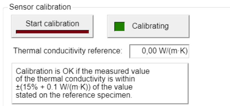
**Figure 4.3.3.1:** The "Sensor calibration" box in the "Settings" tab.
