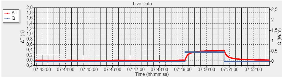
**Figure 5.4.3.1** An erroneous measurement of a material with a low thermal conductivity: the total measurement time was too short. The measurement time is 100 s on low power. The blue line shows the sensor's heater. The red curve the thermopile temperature difference.
