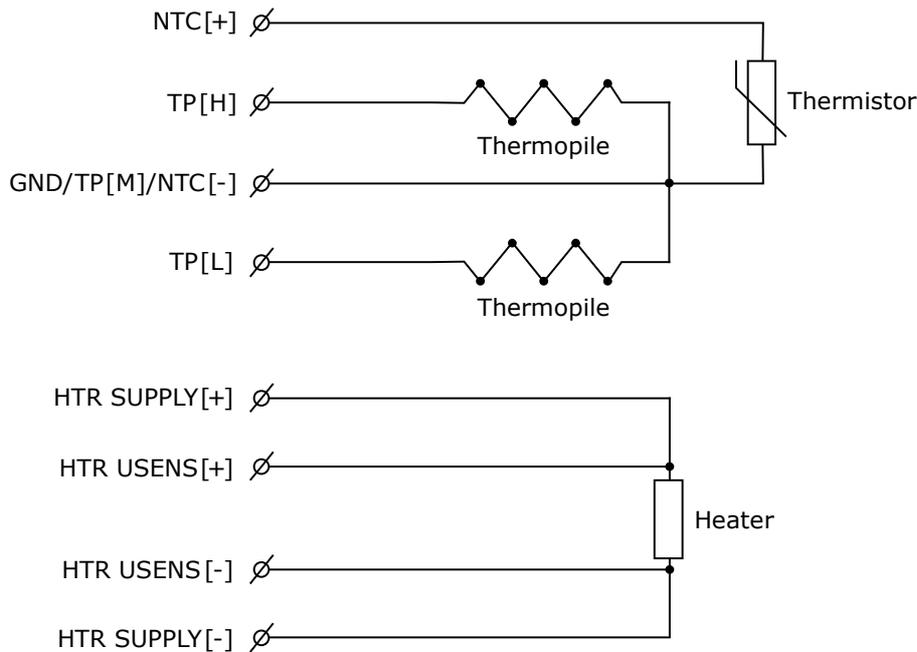
**Figure 7.7.1.1** *Wiring diagram of STP05*
