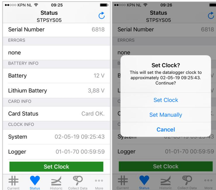
**Figure 4.2.4.2.1** Using the LoggerLink app when setting the STPSYS05 clock over Ethernet
