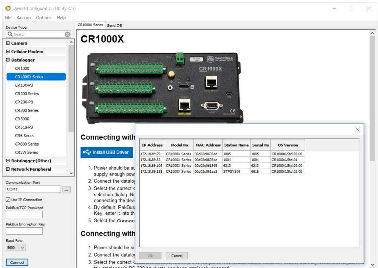
**Figure 7.6.1.1** Using the Device Configuration Utility to find STPSYS05's IP address
