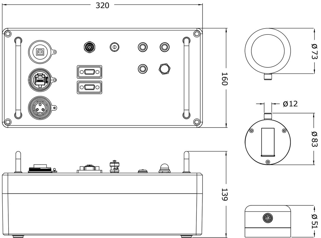
**Figure 3.1.1** Dimensions of STPSYS05 in  $\times 10^{-3}$  m
