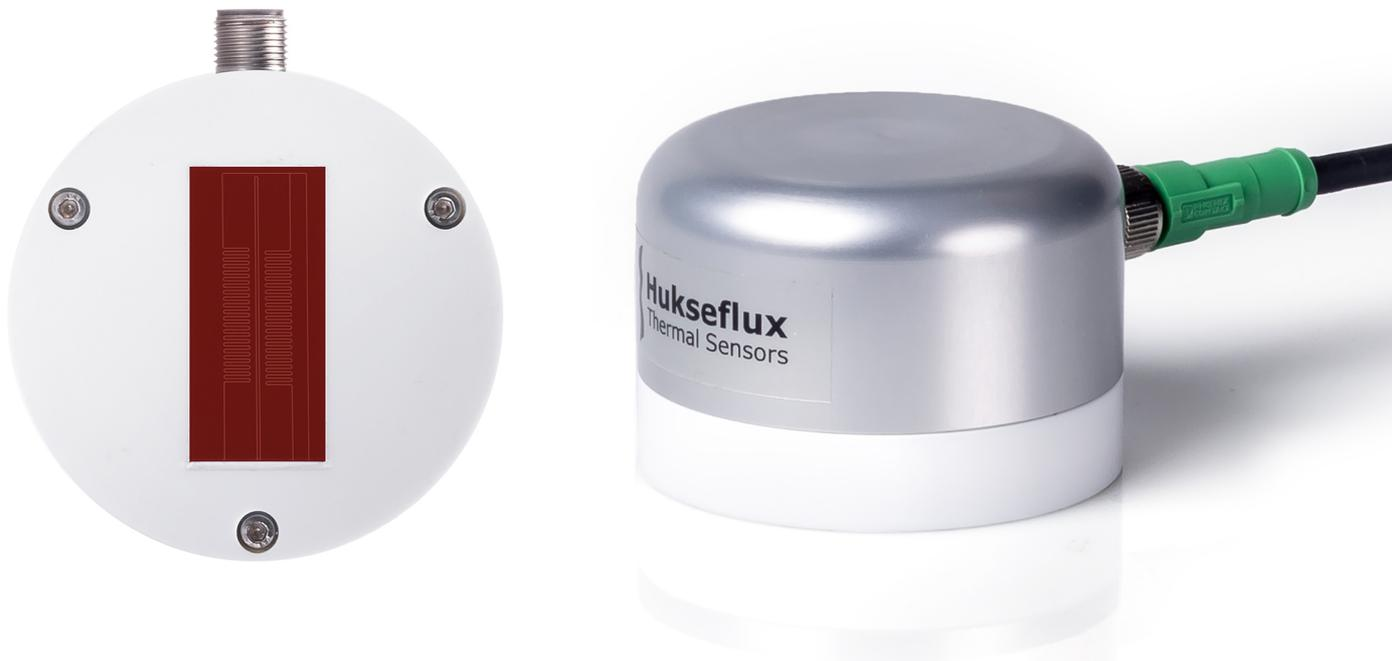
**Figure 0.1** STPSYS05's STP05 sensor, also available as a 'sensor only', is meant for measuring the thermal conductivity of materials at their interface. The bottom view of STP05 on the left shows it is equipped with a heater (line source), a temperature difference sensor (thermopile) and a temperature sensor (thermistor).
