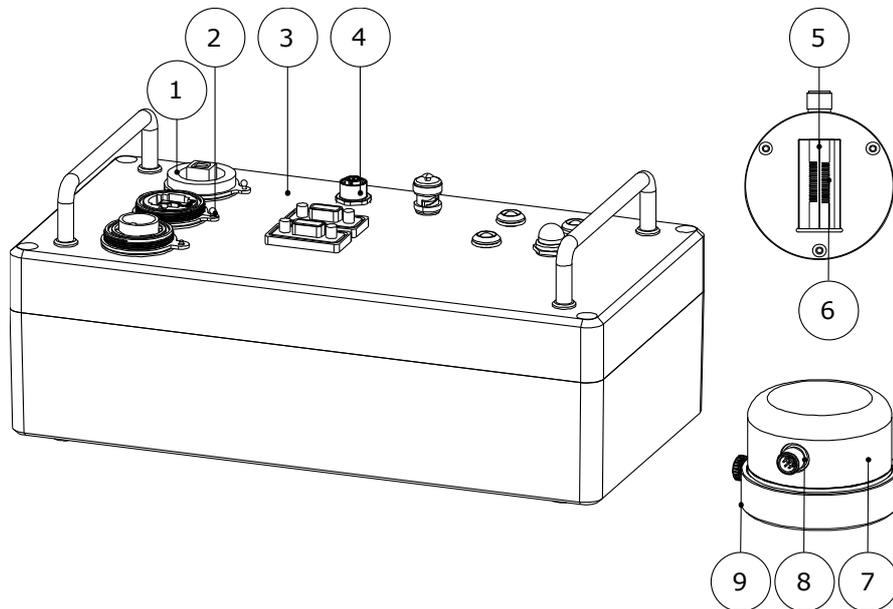
**Figure 0.2** Overview of the STPSYS05 system: (1) USB port, (2) ethernet port, (3) MCU Measurement and Control Unit, (4) connector for STP05 sensor, bottom view of STP05 sensor with (5) heater (line source) and (6) thermopile, (7) body of STP05 sensor, (8) STP05's connector, (9) protective cap
