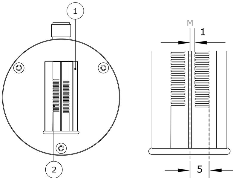
**Figure 2.2.1.1:** Left: schematic of the sensitive surface (bottom) of the STP05 indicating the heater (1) and the thermopile (2). Right: zoom-in on the heater and the thermopile indicating the distance  $y_1$  from the centre of the heater to the hot joint of the thermopile and the distance  $y_2$  from the centre of the heater to the cold joint of the thermopile.
