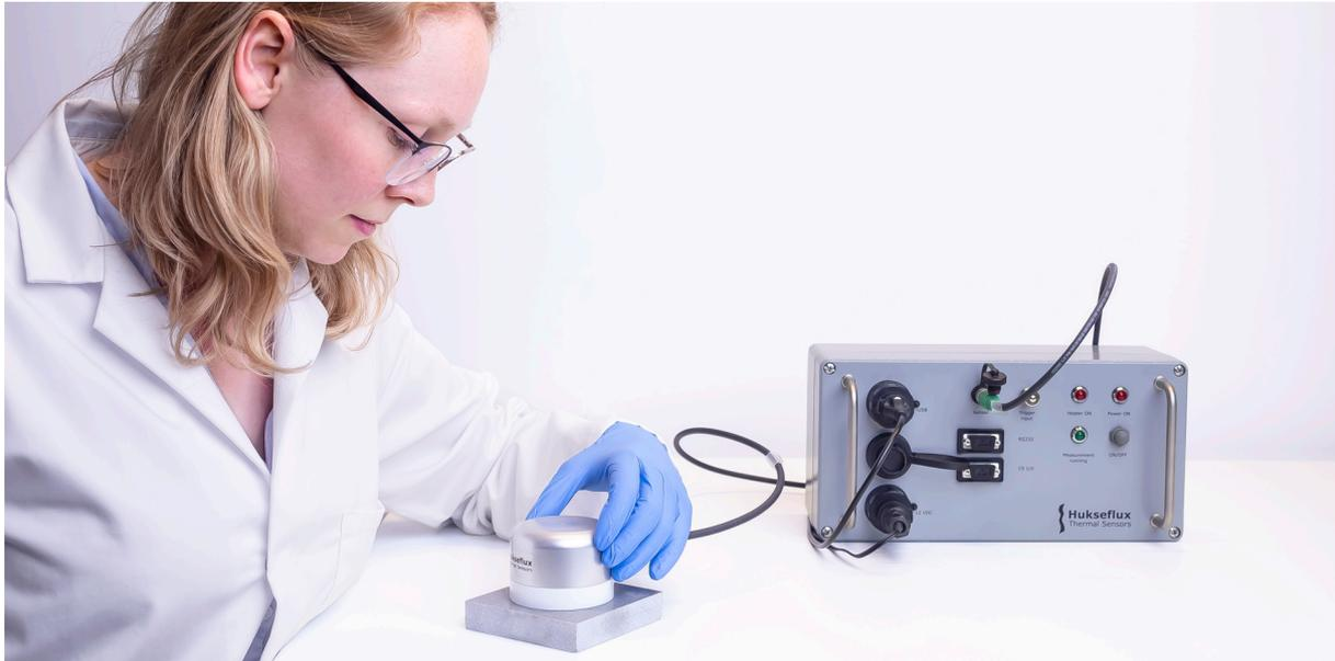
**Figure 0.3** STP05 sensor being applied on a smooth flat surface of a suitable specimen. STPSYS05's MCU performs measurements, data storage and calculation of the measurement result.
