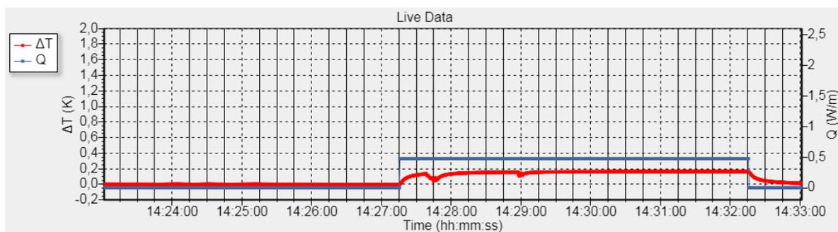
**Figure 5.4.2.1** An erroneous measurement of Pyrex: the sensor moved during the measurement. The measurement time is 300 s on low power. The blue line shows the sensor's heater. The red curve the thermopile temperature difference.
