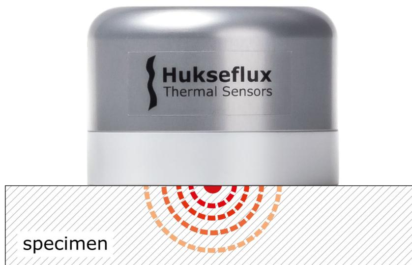
**Figure 2.2.1:** *STP05 with a schematic view of the cylindric thermal field (isotherms). STP05 is conveniently placed at the surface of the specimen, and the heat from STP05's line-source penetrates several millimetres into the material; the measurement is representative for this entire volume.*
