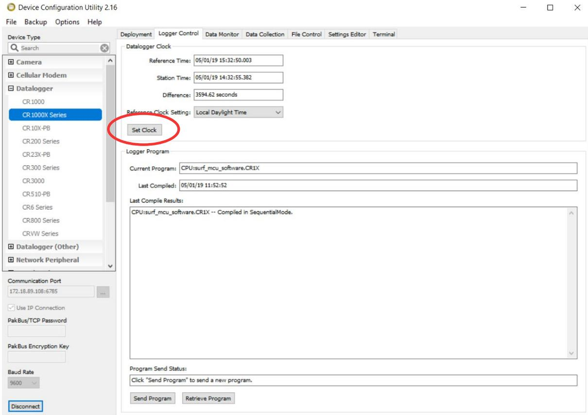
**Figure 7.6.3.1** Using the Device Configuration Utility when setting the STPSYS05 clock via Ethernet
