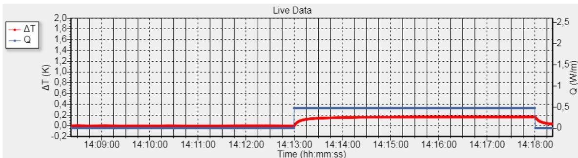
**Figure 5.4.1.1** An exemplary measurement of Pyrex. The measurement time is 300s on low power. The blue line shows the sensor's heater. The red smooth curve the thermopile temperature difference.
