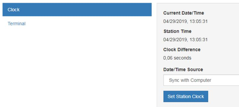
**Figure 4.2.4.1.1** Using the MCU utilities page to set the clock
