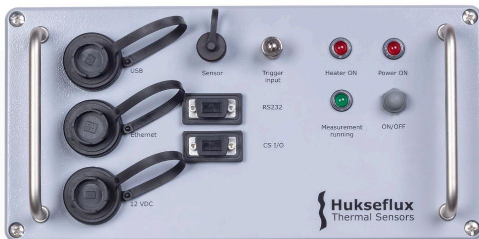
**Figure 2.1.1** STPSYS05's Measurement and Control Unit
