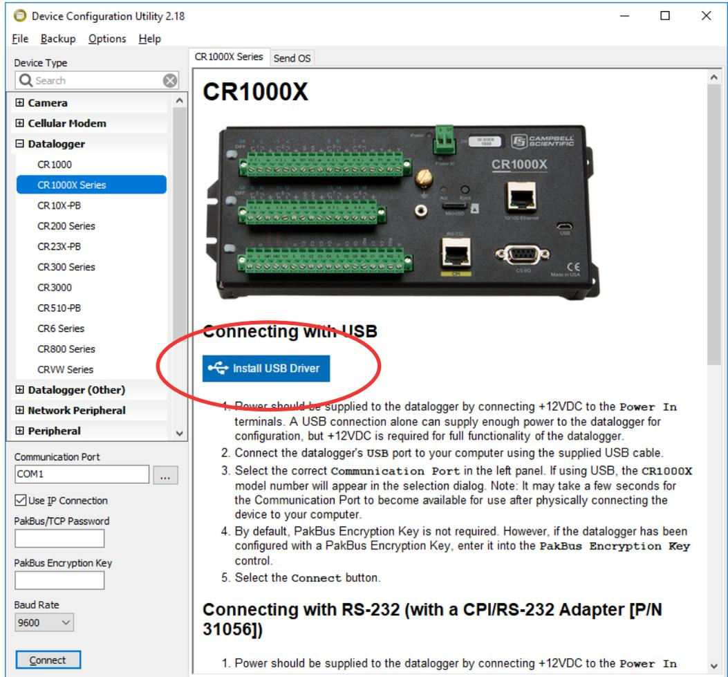
**Figure 7.6.2.1** Using the Device Configuration Utility when drivers are not installed automatically
