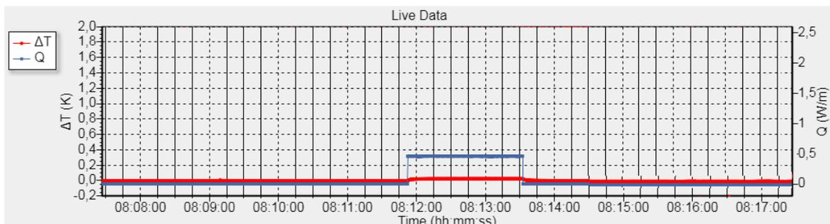
**Figure 5.4.4.4** An erroneous measurement of stainless steel: the heater power setting was too low. The measurement time is 100 s on low power. The blue line shows the sensor's heater. The red curve the thermopile temperature difference.
