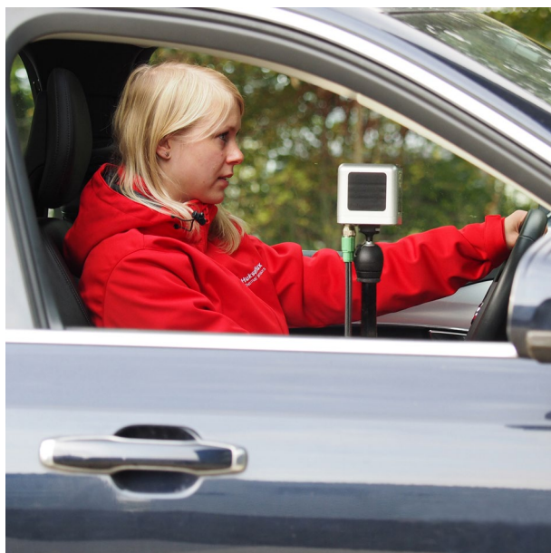
Figure 4 TCOM01 applied in car passenger comfort testing
