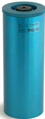
Figure 8 A CRC01 calibration reference cylinder containing a polymethylmethacrylate reference material for calibrating TP02 and TP08
