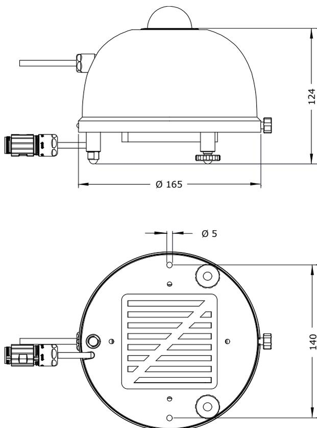
Figure 3 VU01 dimensions in  $\times 10^{-3}$  m.
