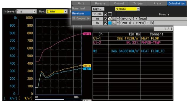
The sensitivity of heat flow sensors is temperature dependent. The FHF05 can measure temperature as well as heat flow. High-precision heat flow measurement is possible by using temperature measured values to perform temperature correction with the LR8450's waveform calculation function.
