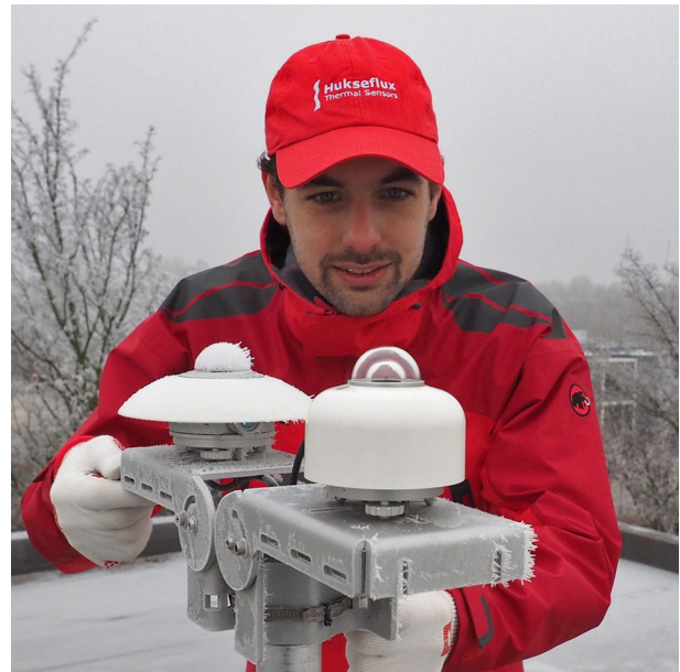
Figure 2 A typical problem in freezing conditions: ice accumulation on the pyranometer dome surface reduces data availability.
