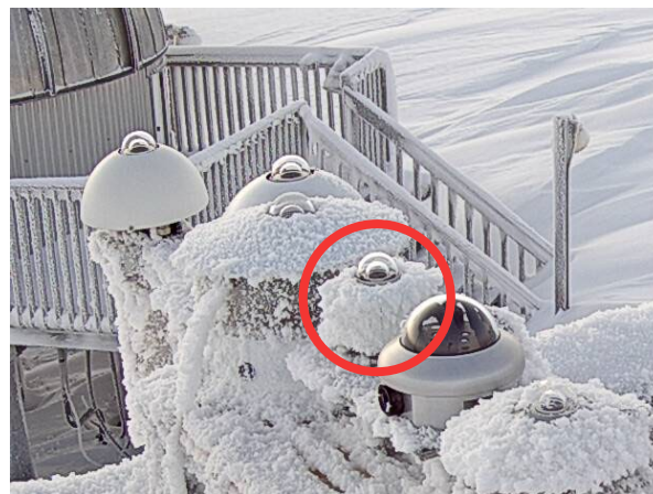
Figure 4 SR30 is battling the elements in Barrow, Alaska: the dome remains ice-free. Note that the neighbouring, completely ice-free sensors are heated with ten times more heating power. Picture taken on 27 JAN 2018 (temperature -30 °C), courtesy of NOAA.
