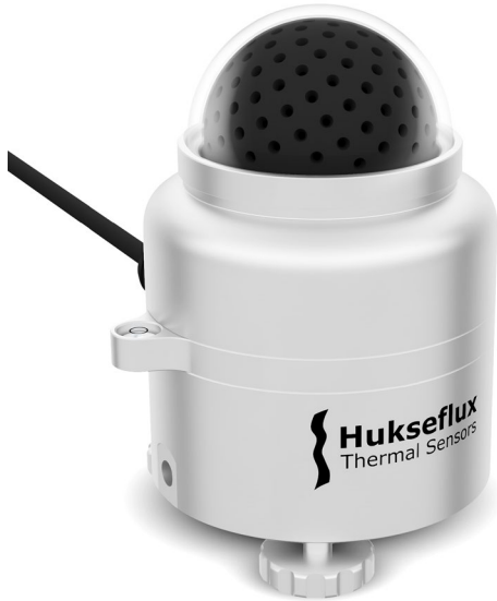
Figure 3 The Hukseflux SRD100-D1 diffusometer, containing a photodiode array with shadow pattern, measures diffuse irradiance without moving parts.
