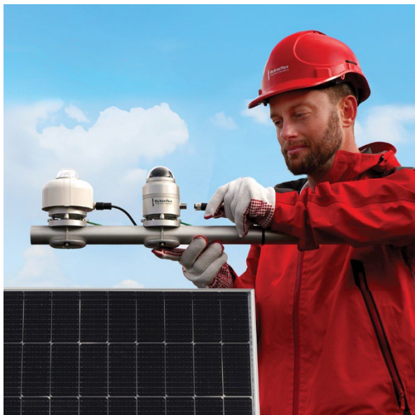
Figure 4 Typical installation of SRD100, next to a normal Class A pyranometer, such as the SR300-D1.
