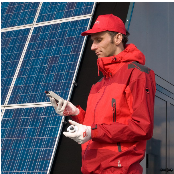
Figure 2 pyranometer in use with LI19 read-out unit
